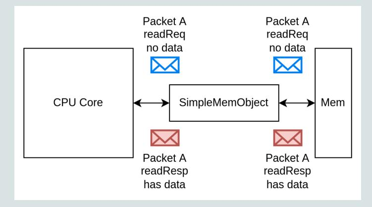
Packets are moved around through ports.
